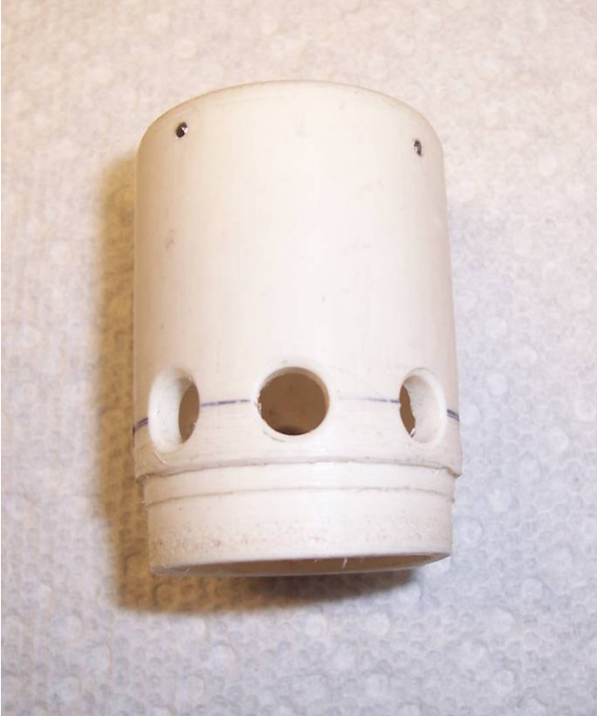
Figure 19 Protective cover for the solid state rectifier made from \frac{3}{4} inch schedule 40 PVC
