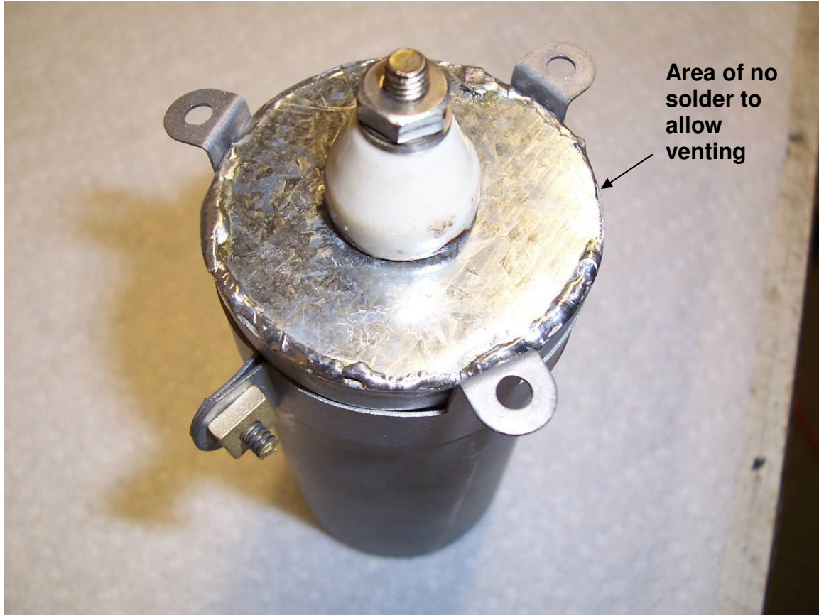
Figure 7 The finished C5 upgrade – note that solder is absent in one small area to allow for venting.
