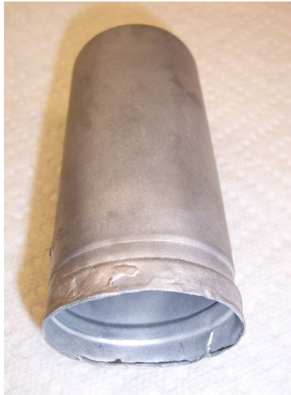
Figure 4 Capacitor C5 housing with contents removed
