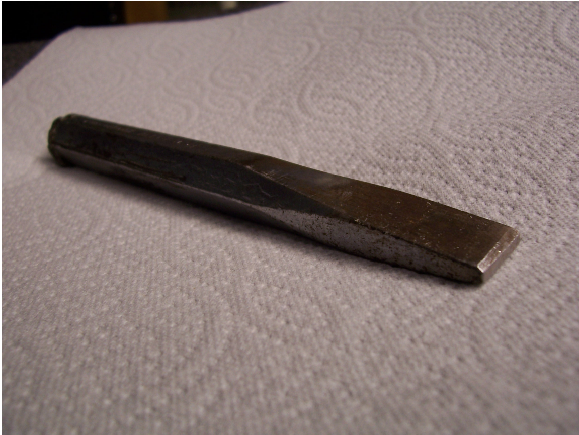
Figure 7: Cold Chisel modified by grinding the end flat.
