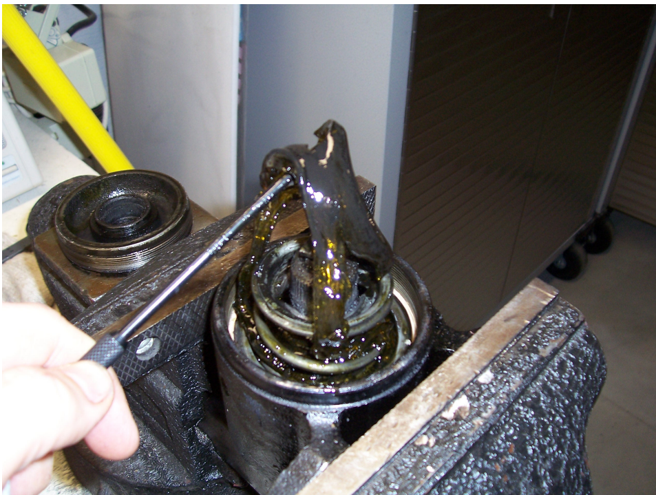
Figure 10 Figure after the housing cap is removed showing the solidified oil with a viscosity similar to that of hot rubber
