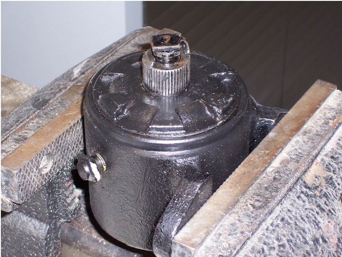
Figure 6 Mounting the damper in a bench vise (adjustment pointer still in place but should be removed prior to removing the end-cap
