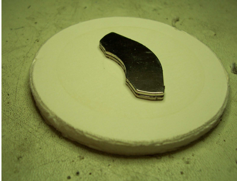
Figure 21 Two rare earth magnets extracted from a failed hard drive stacked together setting on top of a 2.75 inch diameter disk cut from foam board – foam with paper on each side
